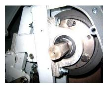
Note: Before tightening the nuts down with a ratchet make sure all four bolts are in. Also the bolts should be tightened down approximately 50-foot pounds of torque
