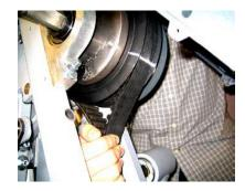
Note: There's two timing marks on the timing belt that's 47 teeth apart from each other, so make sure the top mark on the belt is align with the mark on the Upper Pulley
