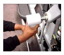
Note: If the Leg Beam assembly has seized and will not come off pulling with your hands, then use a pulley puller to remove the Leg Beam assembly from the shaft.
