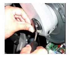
Remove Upper Crank Arm retaining ring
