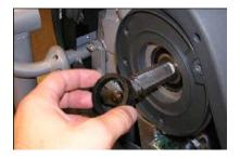
Remove the three idler pulley screws on the Brake Assembly
