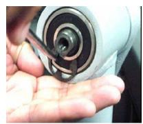
Remove the right Leg Beam by sliding it off of the Upper Crank Arm shaft
