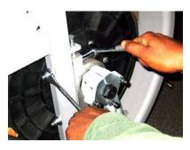
Slide the bolts out and remove the Lower Pulley from the frame
