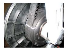
Note: If the timing line on the belt is not aligned with the timing mark on the Lower Pulley, then, hold the timing belt with one hand by the Upper Pulley to prevent throwing the Upper Pulley out of timing. And with your other hand turn the shaft of the Lower Pulley until the timing line on the belt is aligned with the mark on the Lower Pulley.
