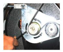
Loosen the Brake tension bolt approximately thee complete turns
